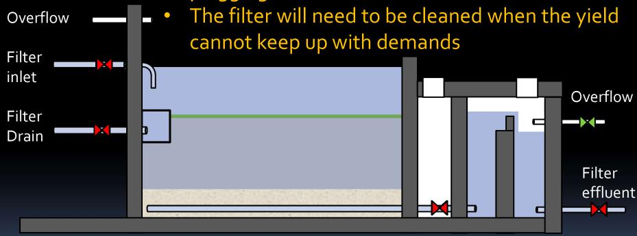
What goes into the filter will go out of the filter (Excess can be overflowed if needed)
